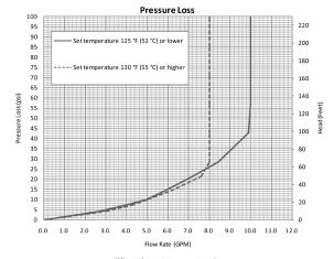
When the set temperature is 130 °F (55 °C) or higher, maximum flow rate is limited to 8.0 GPM.
