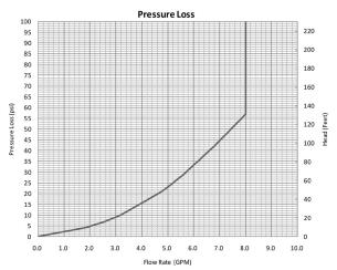
Flow rate is limited to 8.0 GPM.
