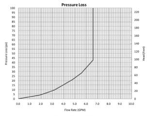
Maximum flow rate is limited to 6.6 GPM.
